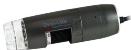
FIGURE 1. Instrument for optical microscopic imaging (Dino-Lite AM-311s USB Microscope 10× - 200× coupled with 5 high intensity LED)
